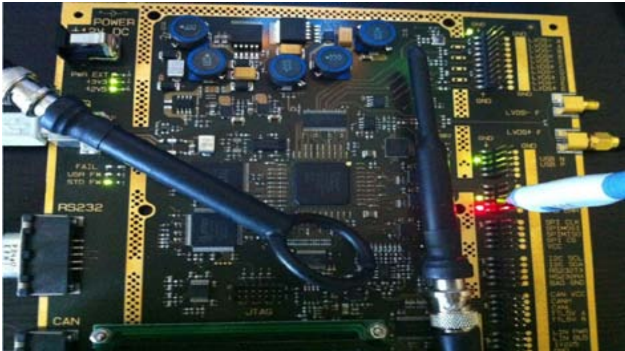
Figure 2 Rohde & Schwarz offers a family of near-field E and H field probes (or “sniffer” probes R&S®HZ15) which can be used to diagnose the cause of an electromagnetic interference problem.
