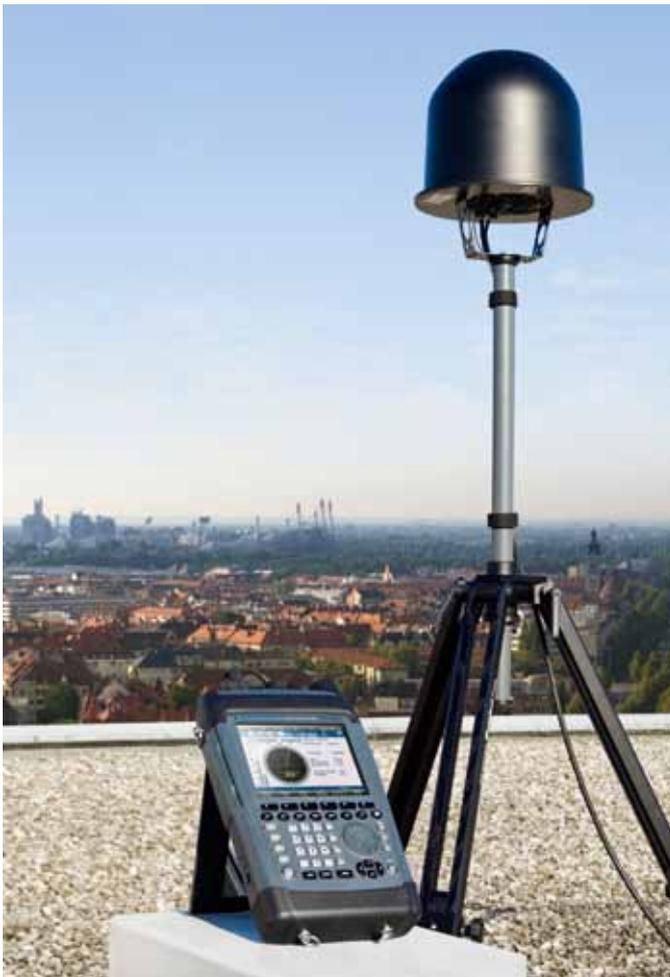
Due to the lithium-ion battery pack built into the R&S®DDF007, the DF station does not require an external power supply. If the operating time in DF mode exceeds two hours, it can be extended using additional battery packs.
