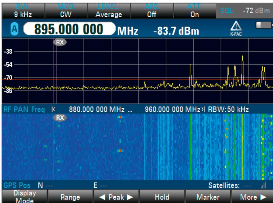
been reduced and the resolution increased. The waterfall display shows the interfering signal's behavior versus time and makes it possible to measure the transmit duration.
