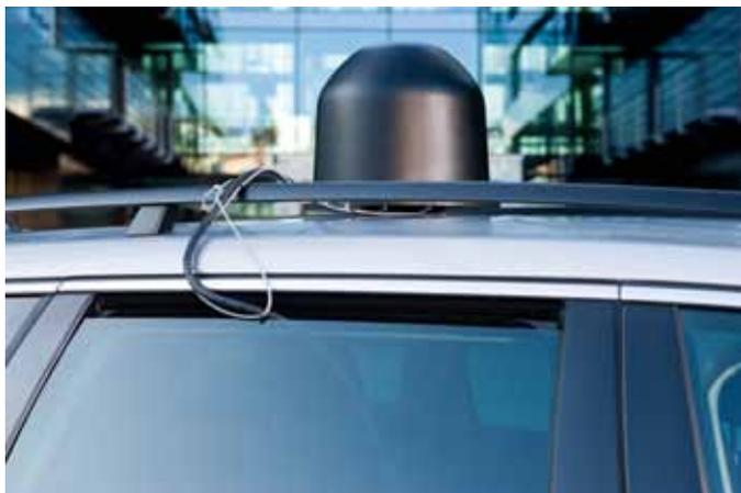
For added safety, the DF antenna is also secured with a steel wire, which can be attached, for example, to a handle inside the vehicle. The DF antenna cable set is routed into the vehicle through a slightly opened window and is connected to the R&S®DDF007 (see photo at bottom of page 3). If necessary, the direction finder can be supplied with power from the cigarette lighter via the R&S®HA-Z202 vehicle adapter.
