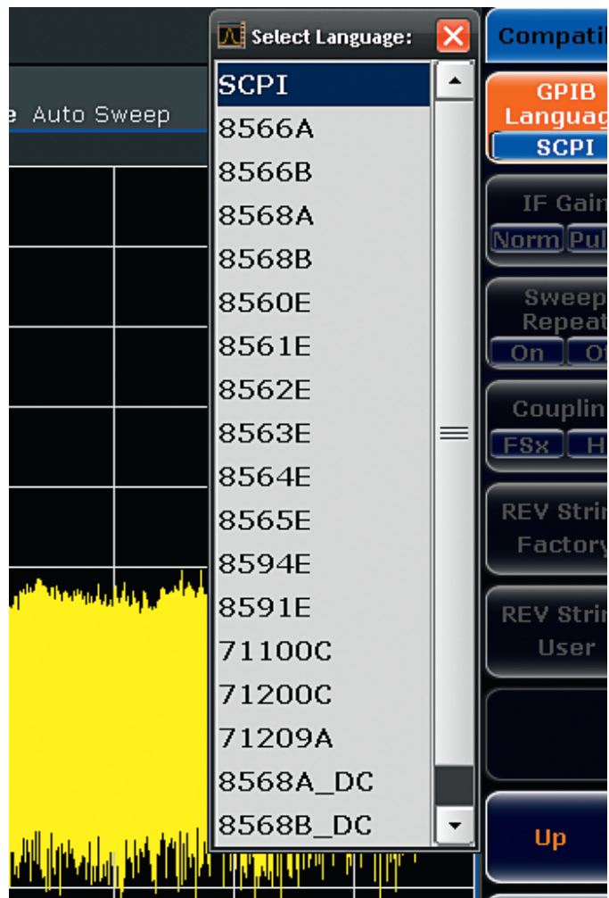
FSV emulation mode: selection of analyzer to be emulated by the FSV
