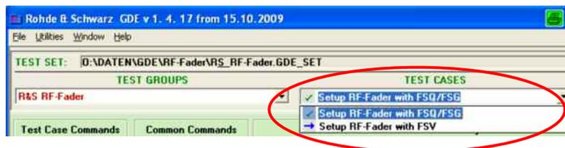
6. Modify Test Case parameters such as the frequency and level via the user interface. Default values are 310 MHz for FSQ/FSV center frequency and SMU output frequency, a FSQ/FSV reference level of 0 dBm and a SMU Level of 0 dBm.
