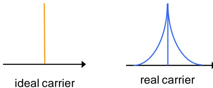
**Figure 4.** An ideal carrier would have no phase noise, however a typical carrier will have skirts whose amplitudes generally follow  $(1 / f)$  distribution.
