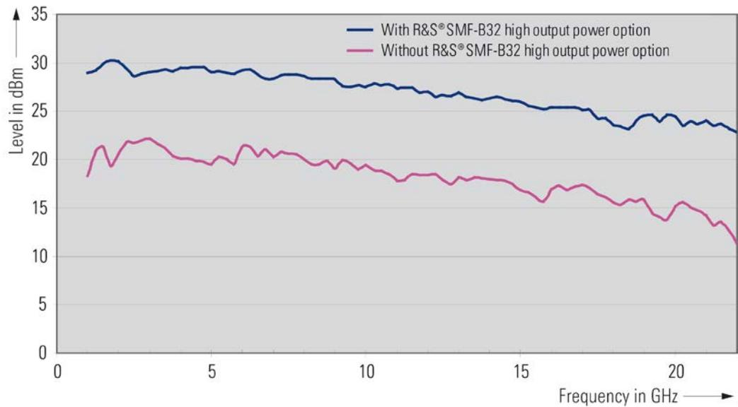
**Figure 3. Actual maximum output power of a signal generator is often found in the products data sheet. Example of the R&S®SMF with and without the high output power option in the frequency range 1 GHz to 22.**
