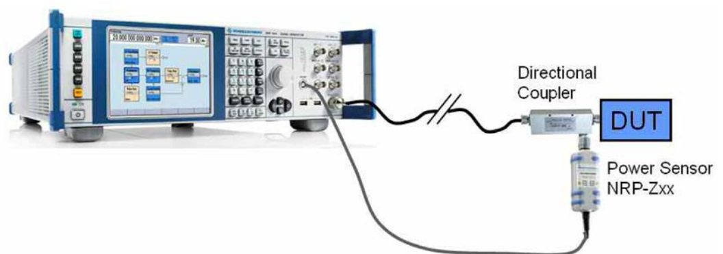
Figure 11. Scalar measurements can be carried out using a signal generator and a power sensor for a more cost-effective solution than the use of scalar network analyzer.
