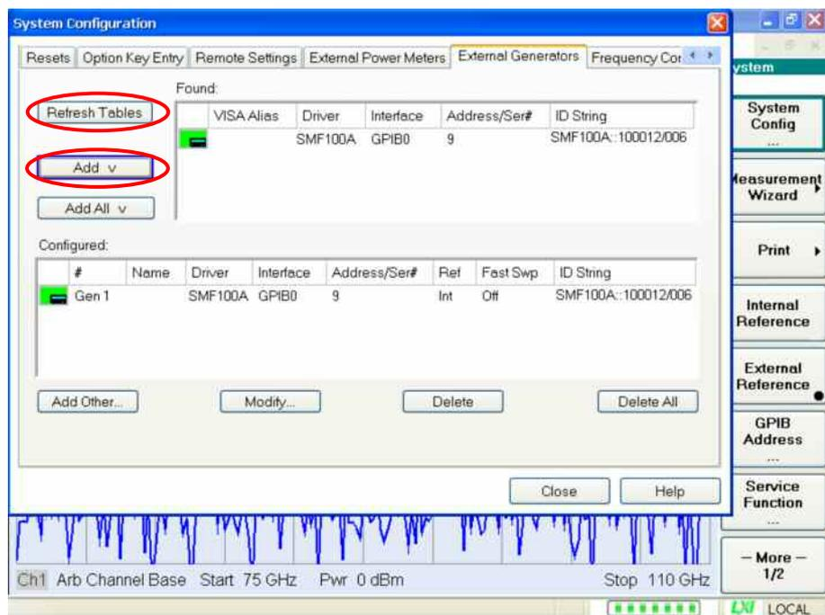
Fig. 4.13: Detecting and adding an external generator
