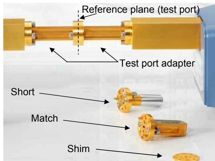
Fig. 4.6: (Direct) Through and other calibration standards
