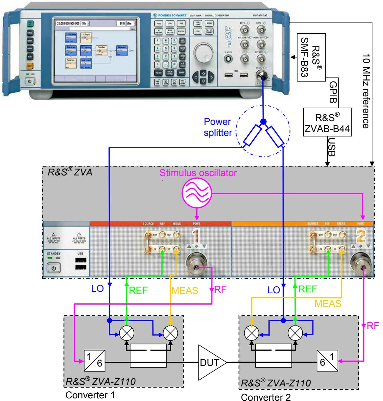
Fig. 4.14: Test setup with an external LO generator
