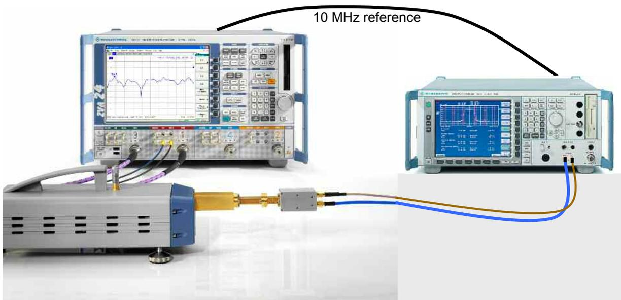
Fig. 4.10: Test setup for measuring the RF matching of the R&S® FS-Z110 mixer
