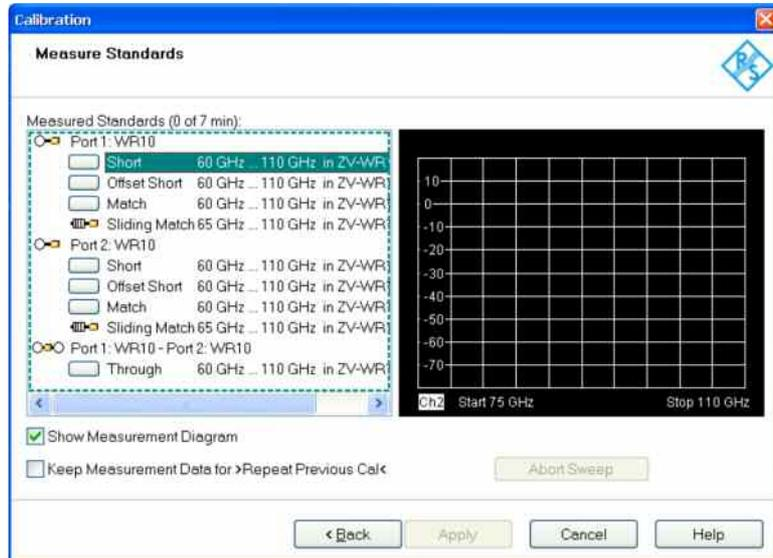
Fig. 4.7: Calibration dialog: TOSM calibration using the R&S® ZV-WR10 calibration kit
