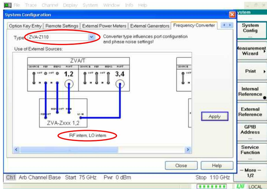
Fig. 4.2: Configuring the converters on the R&S® ZVA
