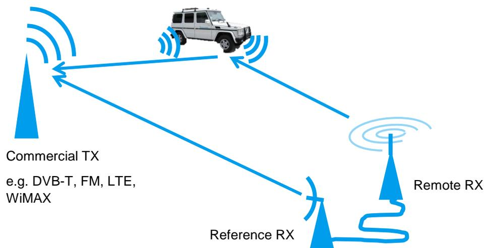
Figure 4-9: Passive Radar
