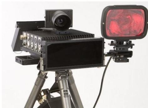
**Figure 4-4: Mobile traffic monitoring radar, MultaRadar CD – Mobile speed radar for speed enforcement from Jenoptic**
