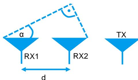
Figure 4-10: Mono-Pulse Technique (Phase)
