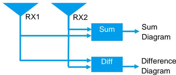
Figure 4-11: Mono-Pulse Technique (Amplitude)
