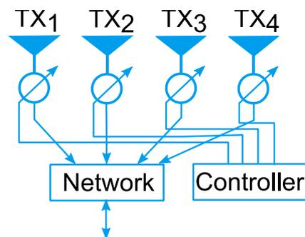
**Figure 4-13: Basic Principle of DBF**
