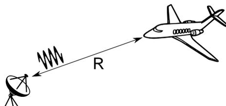
**Figure 4-2: Pulse radar principle.**
