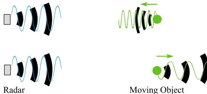
**Figure 4-1: Principal operation of radial velocity measurement.**
