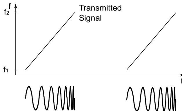
Figure 4-3: Pulse Compression Radar using LFM.
