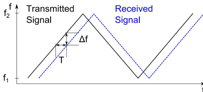
Figure 4-5: Basic principle of FMCW radar.
