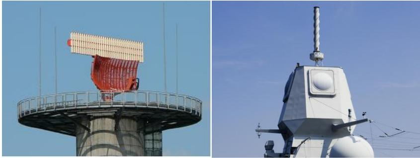
**Figure 4-12: 360-degree rotating antenna (left) of an air surveillance system and electronically steered antenna (right)**
