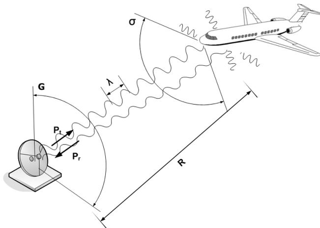
Figure 3-1: Radar principle
