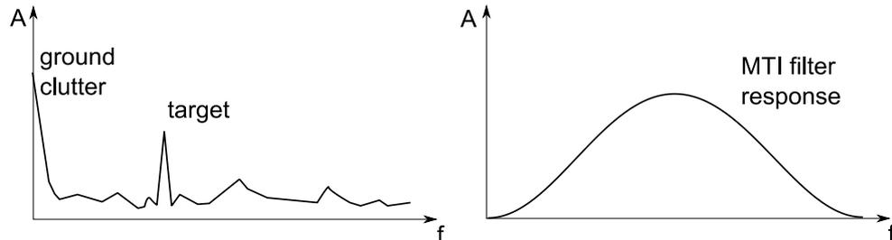
Figure 4-7: Radar echo and MTI filter response
