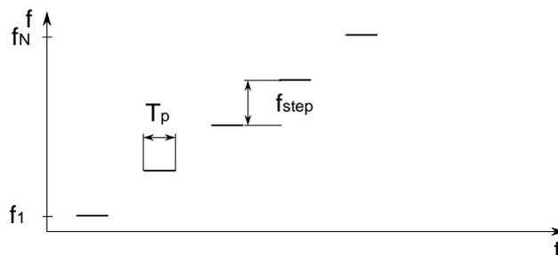
Figure 4-6: Stepped Frequency Radar
