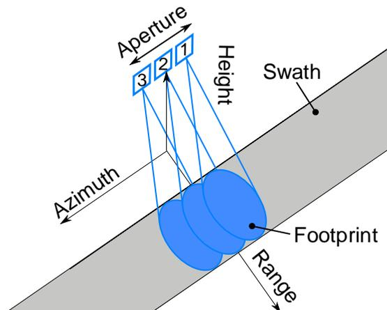
Figure 4-8: Synthetic Aperture Radar (SAR)
