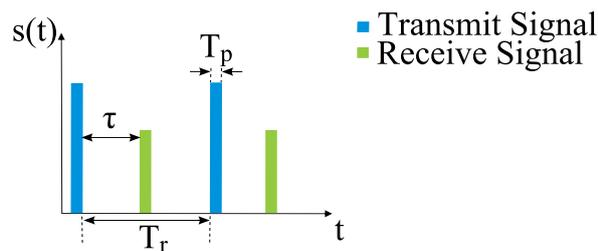
**Figure 3-1: Radar principle.**
