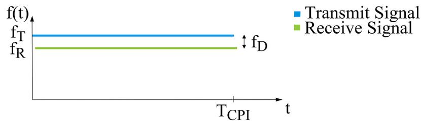
Figure 4-1: Monofrequent Continuous Wave radar.
