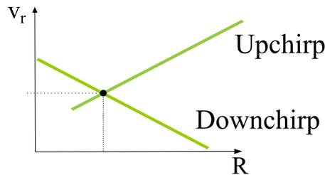
Figure 5-2: Interception between Up- and Downchirp Radar Echo Signals.
