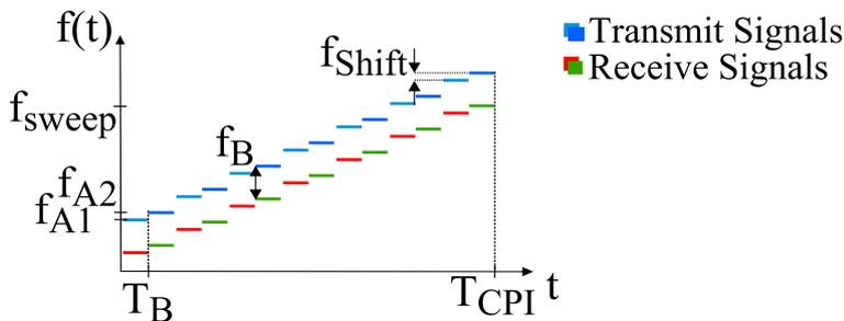
Figure 5-4: Multiple Frequency Shift Keying.
