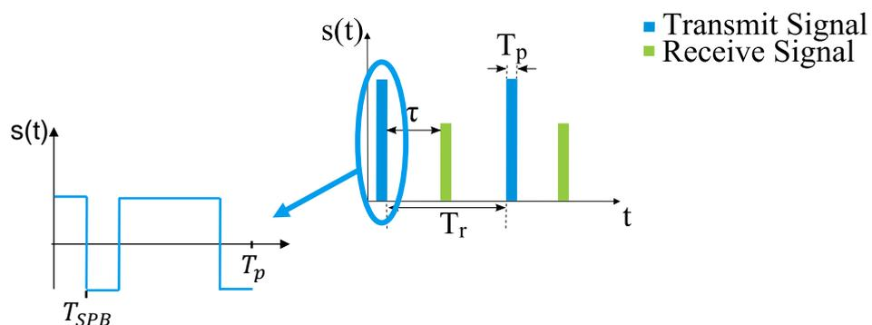
**Figure 3-3: Pulse compression in a single pulse.**
