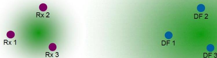
Fig. 10: The areas (green fields) where good geolocating results can be expected: TDOAs left and DF stations right.
