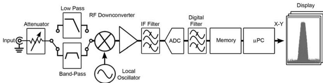
**Figure 2** Basic Block Diagram of Digital (stepped) RF Measurement Instrument
