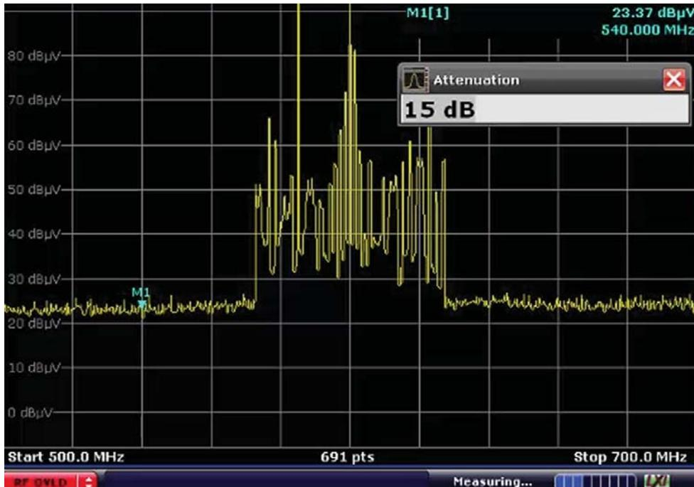
Figure 5 Overloaded signal conditions during a wideband scan
