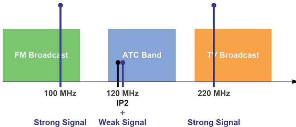
Figure 3 Challenging real world environments dictate RF performance requirements
