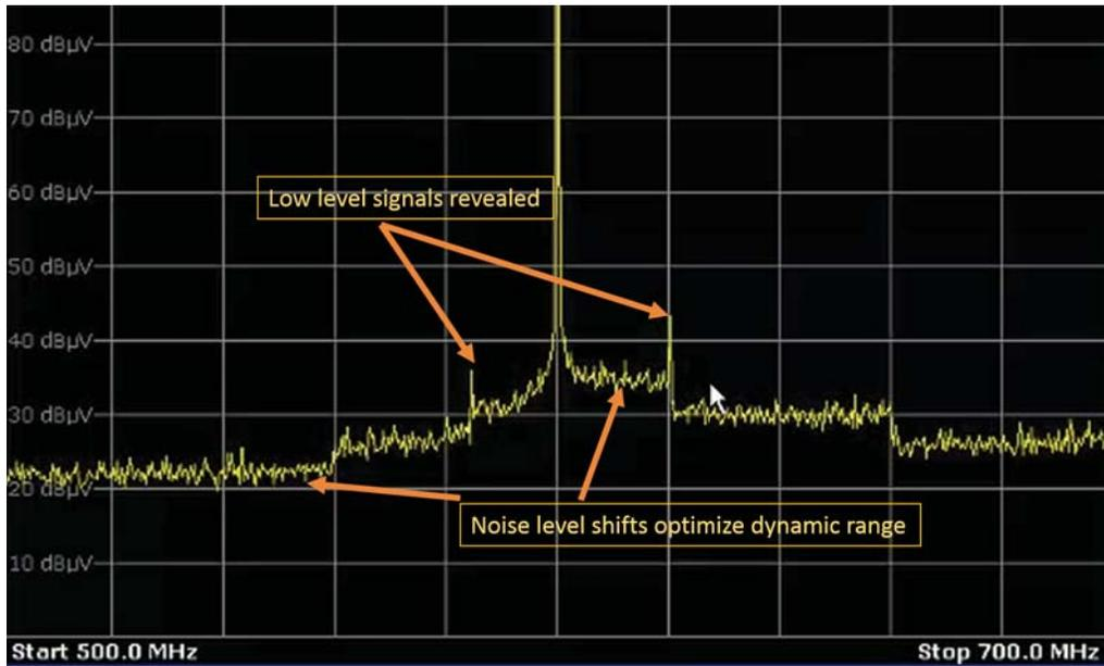
Figure 7 Automatic Gain Control
