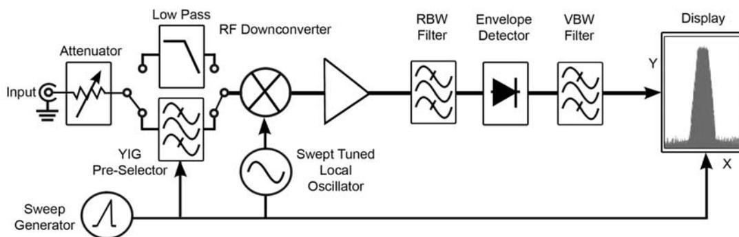
Figure 1 Block Diagram of an Analog (swept) RF Measurement Instrument
