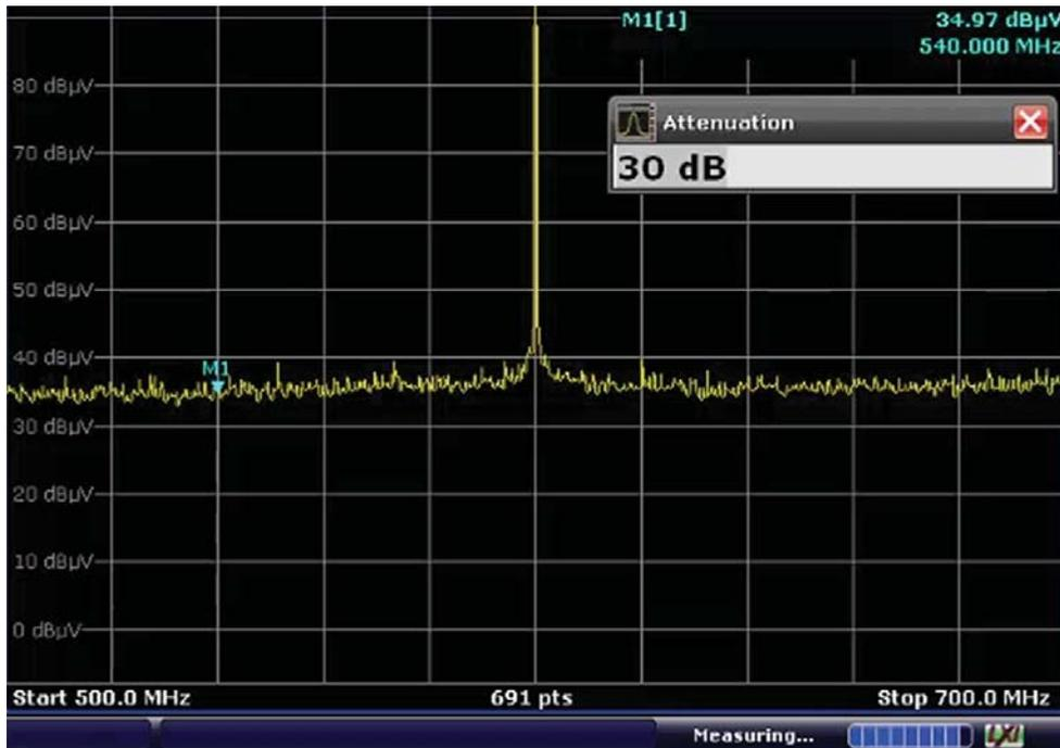
Figure 6 Attenuation adjusted to 30 dB to remove overload condition
